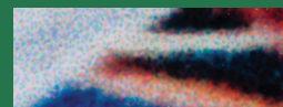
Inkjet dots formed by the application of liquid ink to the surface of paper
